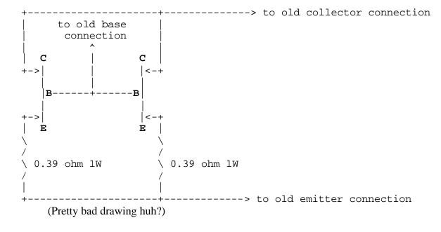
The 0.39-ohm resistor allows the transistors to be hooked in parallel without one transistor going into thermal runaway and trying to drive the whole load itself. (A good place to find out more about hooking transistors in parallel is a Voltage Regulator handbook of some kind)
